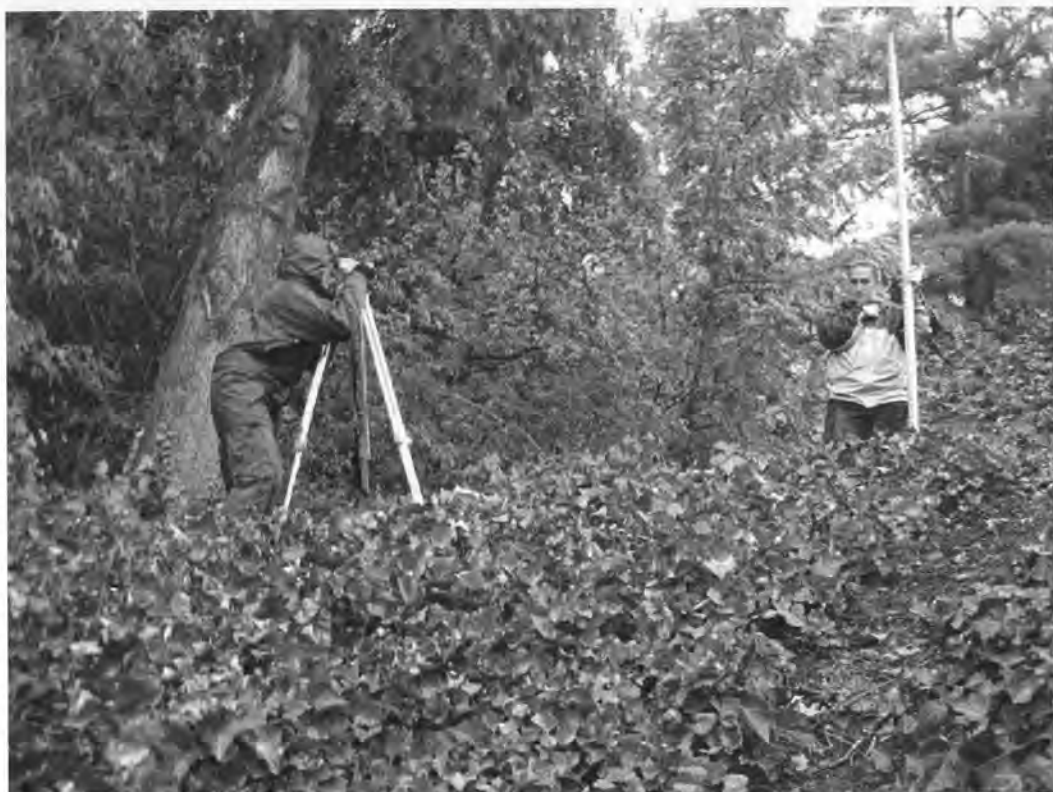
Conducting cross-section surveys as a field work component for LA227, 2004. Photograph by Shannah Anderson.
